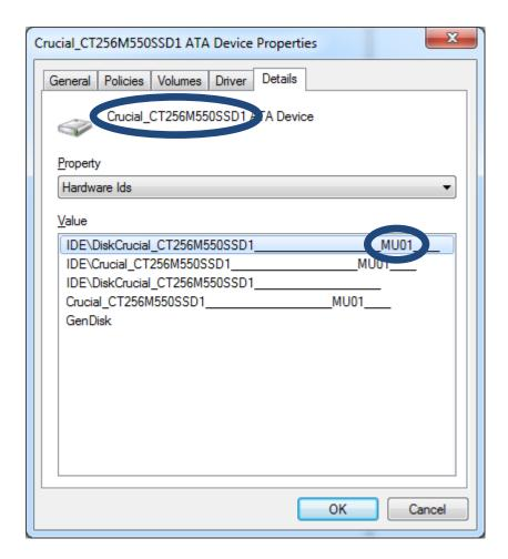
The drive model and current firmware are circled in the example above.
